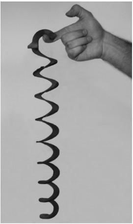
If the boiler was from any reason operated in incorrect way, it is possible, that the turbulators were clogged and thereby the flue gas transition was decreased. In this case it is necessary to demount turbulators and to clean the space between particular threads, for example by wire brush. Put the turbulators back into the pipes, not to decrease efficiency of the boiler. (This is not related to the 15 DPX model).
