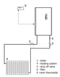
In case that you use the room thermostat in your heating system the regulation of heating water temperature is controlled similar till the moment when the request for heating is terminated (the temperature set on the room thermostat is fullfiled and the room thermostat is switch off).
